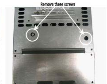
Figure 5.h - Changing of EMC protection class, MF6
