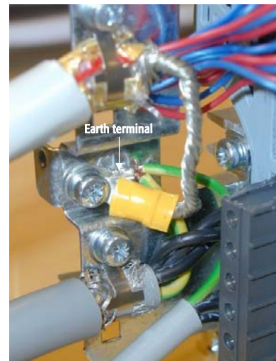
Figure 6.g - Cable installation in Carel NXL, MF2 (500V, 3-phase)
